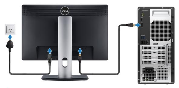
() NOTE: The location to connect the display cable can vary if your computer has a discrete graphics card installed. For optimal graphics performance, ensure to connect the display cable to the graphics card if there is one installed.
