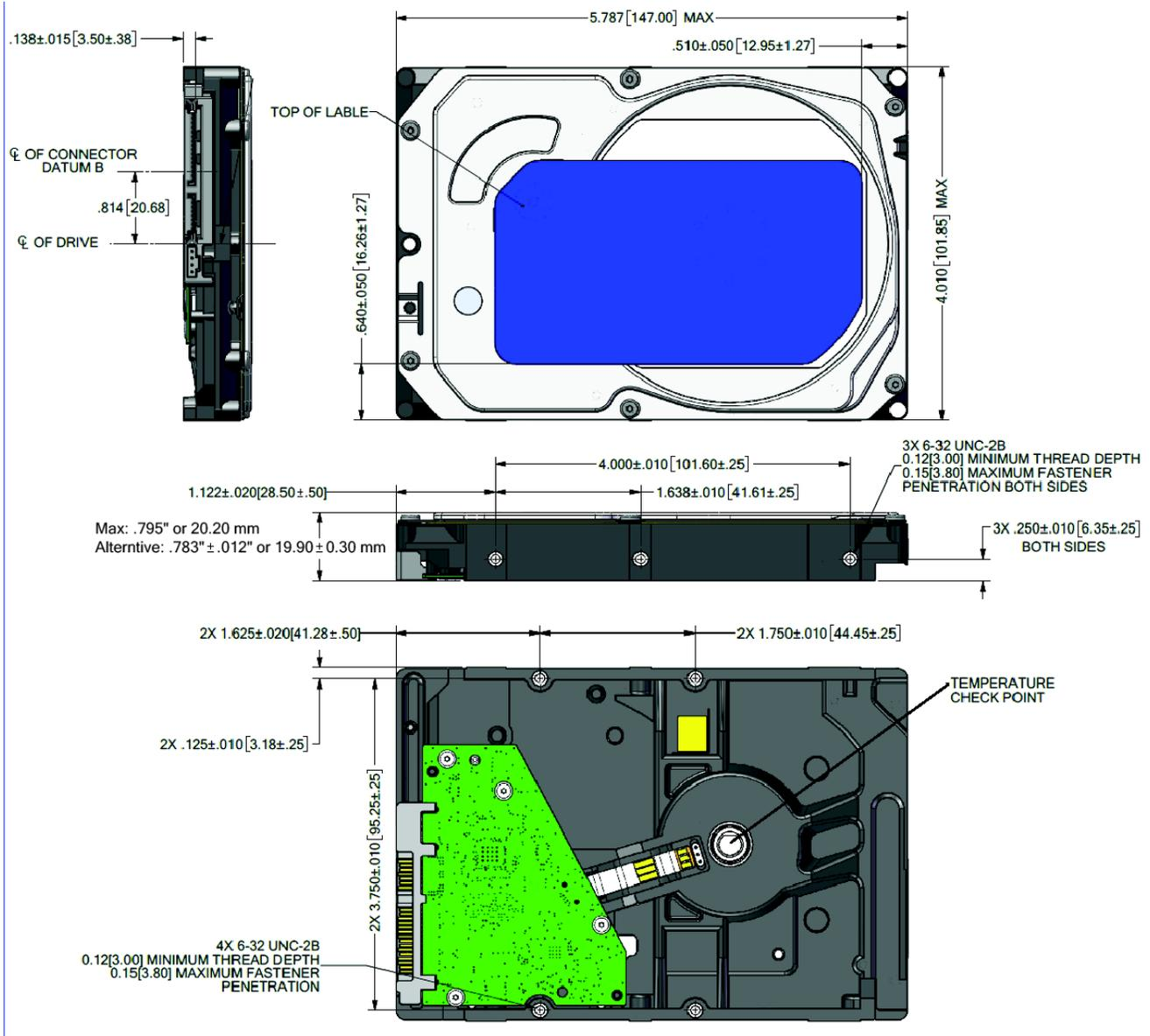
Figure 5 Mounting dimensions (ST2000VN004 model)
