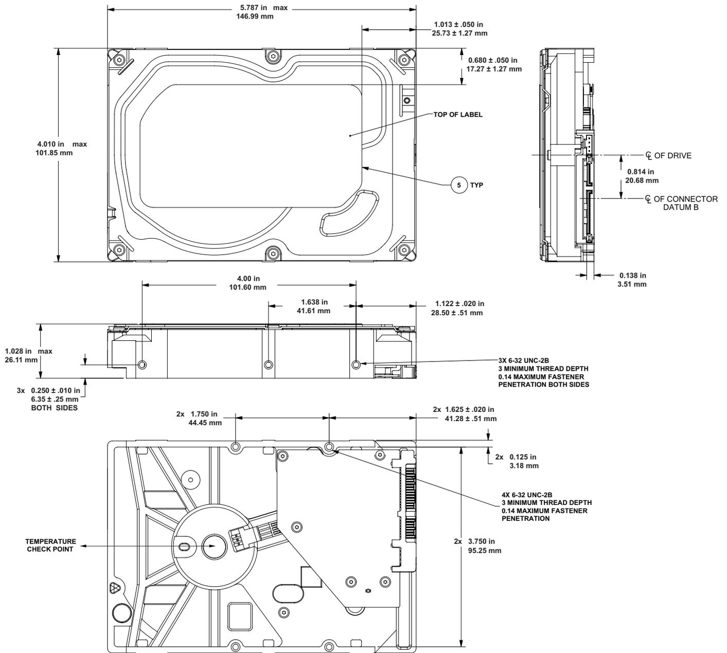
Figure 7 Mounting dimensions (ST8000VN002 & ST6000VN006 models)
